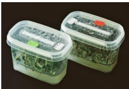
Fig 1: Microbox, provided with hermetically closed cover and breathing strip
